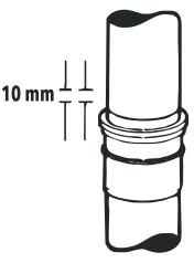
WITHDRAW PIPE (10 MM). THIS WILL ALLOW FOR EXPANSION. ALL FITTINGS MUST BE SUPPORTED BY A BRACKET WHEN INSTALLED VERTICALLY.
