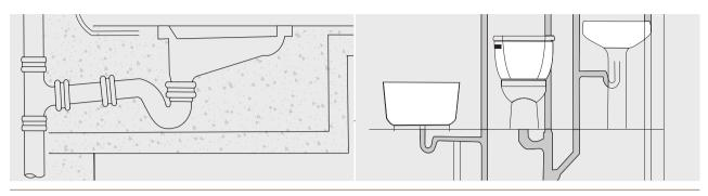
Traps are very important parts of drainage and sewage system and are most critical to ensure efficient working of the system. Traps prevent foul gases or air to enter back in passage and at a same time allow waste to flow through them.
